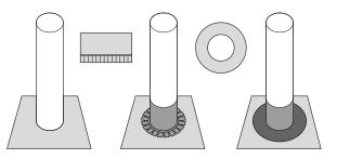
Cut flashing strips at regular intervals of approx. 30 mm and guide them around the pipe. Slip a ring segment over the pipe and bond it to the substrate.
