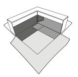
The first flashing strip must be laid with an inverted pleat.
